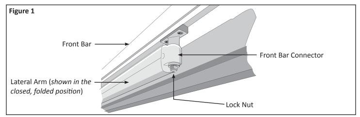
Note: The two Front Bar Connectors attach each Lateral Arm, left and right, to the Front Bar.
