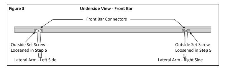
6. Have your helper move and HOLD both Lateral Arms (AT THE ELBOWS) to the desired location (SHOULD BE APPROXIMATELY 2 INCHES FROM THE SQUARE BAR). The loosened Front Bar Connectors will realign themselves during this process.
